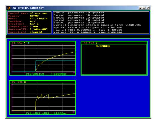
The first scope (SC1) shows the throttle rising to a maximum value of 100 and the vehicle speed gradually increasing. The third scope (SC3) shows the vehicle RPM. Notice the changes in the vehicle RPM as the gears shift from first to fourth gear as displayed in the third numerical scope (SC2).
